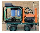
The Wavecleaner VAC is fully portable and mounted within a sturdy cage and operates using a 12vDC rechargeable, hi-capacity battery pack, Similar in appearance to a small gen set, it can be permanently or temporarily sited on a standard marina trolley, or similar, enabling easy and fast access for just one operator to the area of the spill.
