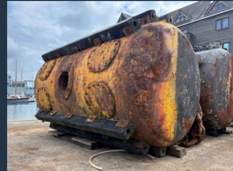
The old post-WW2 Admiralty steel mooring buoys have reached the end of their operational life. Photo – Falmouth Harbour.
